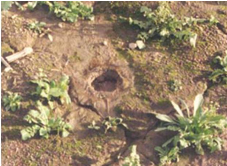
Figure 10. Example of Chimney Effect
