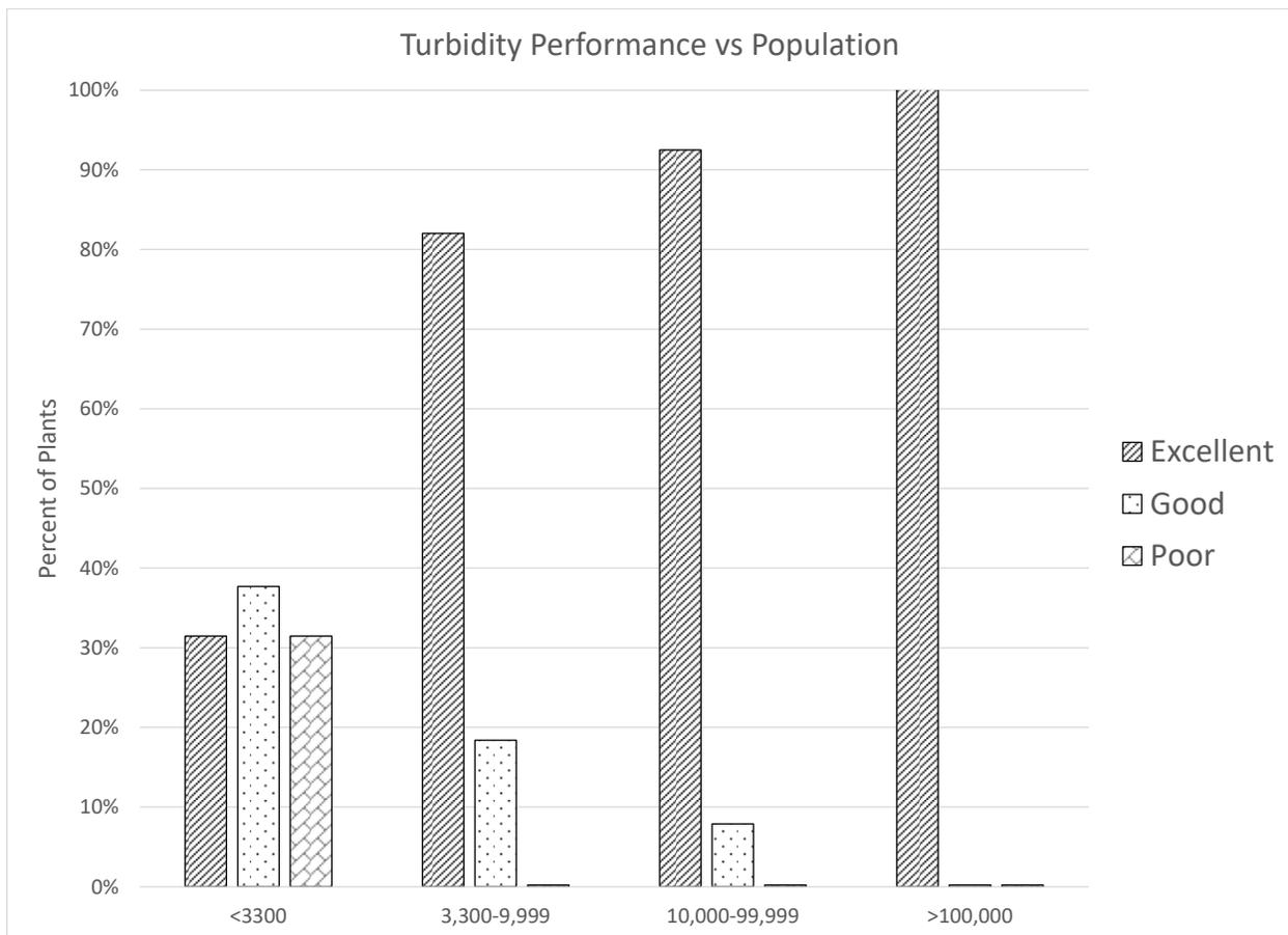
**Figure 11-1:** Rapid Rate Filtration Turbidity Performance in Washington, 2017.
