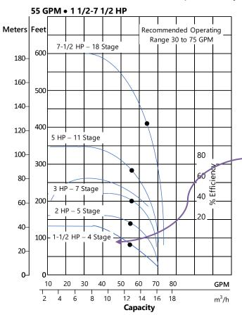
The figure at left is a family of pump curves, beginning with a  $7\frac{1}{2}$  hp pump (top) down to a  $1\frac{1}{2}$  hp pump (bottom).
