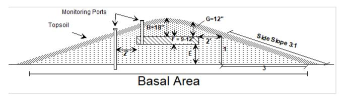
Note: the distance between the outer edge of the mound and the bed is 2 feet. On a level site, there is no "D"
