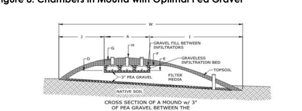
Field experience has shown that a 2-4 inch later of pea gravel at the mound/soil interface may inhibit capillary action. (Adolfson Associates, Inc. 1999)
