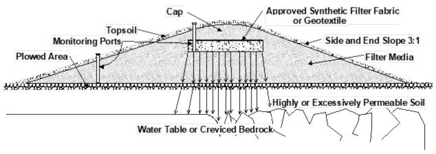
Figure 4. Cross-Section of a Typical Mound System Showing Effluent Movement in a Slowly Permeable Soil on a Sloping Site
