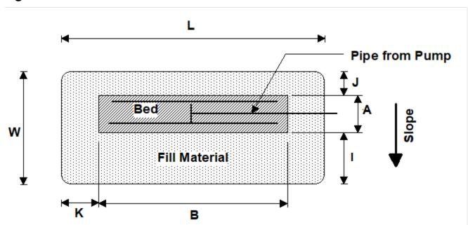
Figure 10. Plan View of Mound and Basal Area for Filter Media
