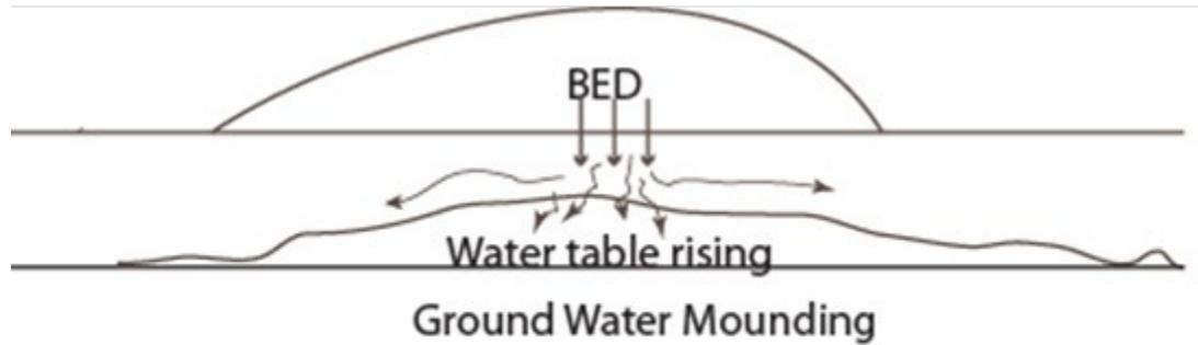
The water accumulates under the bed area faster than the soil can disperse it laterally
