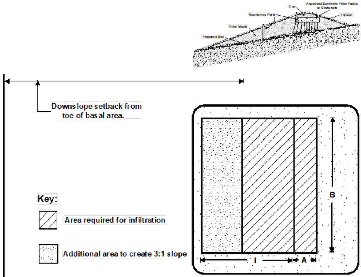
**Figure 6. Detailed Plan View of Filter Media and Available Basal Area on Flat and Sloped Sites**
