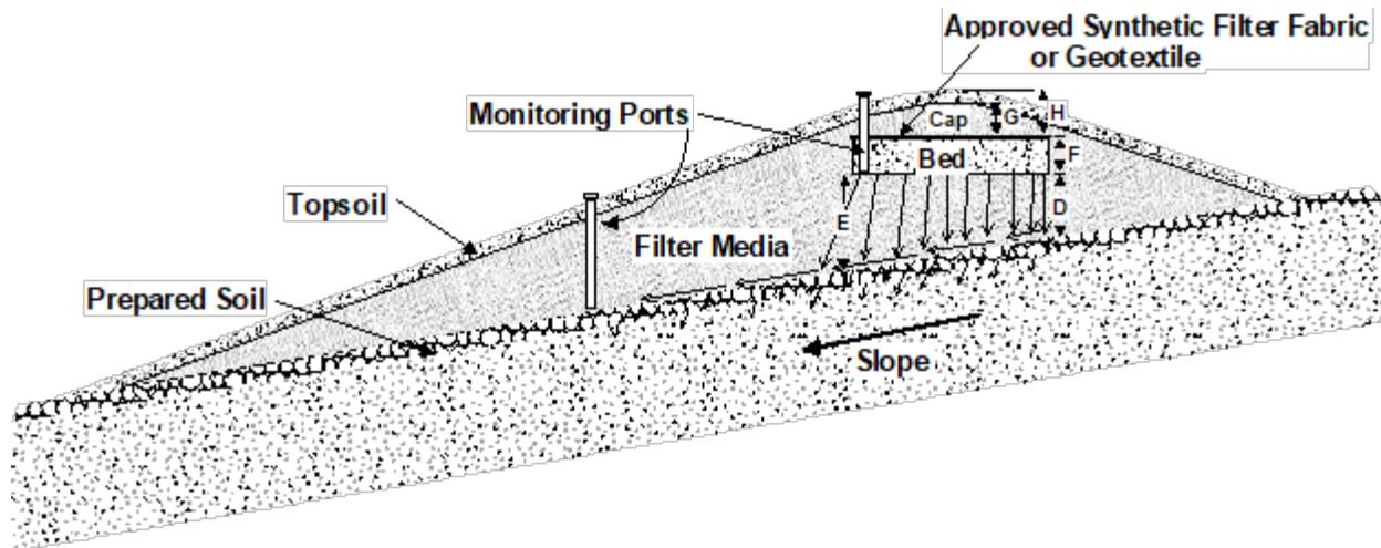
Figure 10. Plan View of Mound and Basal Area for Filter Media
