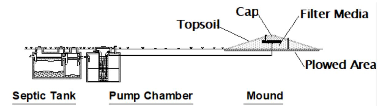
**Figure 3. Cross-Section Showing Effluent Movement in Permeable or Excessively Permeable Soils (Type 1 Soils)**
