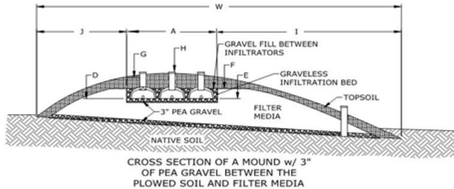
Field experience has shown that a 2-4 inch later of pea gravel at the mound/soil interface may inhibit capillary action. (Adolfson Associates, Inc. 1999)
