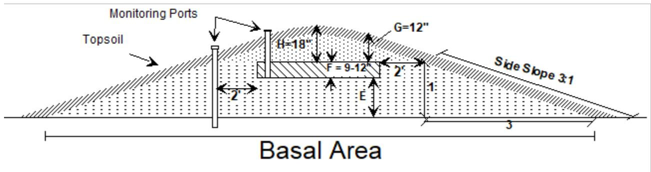
Note: the distance between the outer edge of the mound and the bed is 2 feet.
