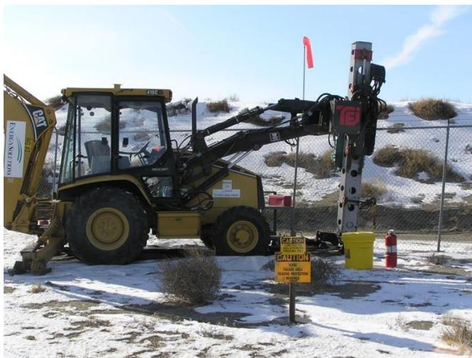
**Figure 4. Drill Rig**
