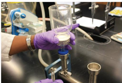
An SPU lab analyst prepares to conduct a membrane filter test in their microbiology section. Photo courtesy of Seattle Public Utilities
