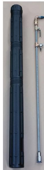
Sampling station rods easily thread onto a spring-loaded sampling tap, reducing your chance of obtaining an unsatisfactory water sample.
