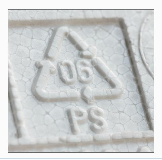
Expanded polystyrene (EPS) is a lightweight material that is made when polystyrene beads are expanded during processing and placed into molds to create products.
