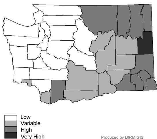
To control radon in new construction in those counties known to have high or very high radon potential, the Washington State Building Code (see Technical Notes) requires underslab venting, which reduces the infiltration of radon gas into buildings.
