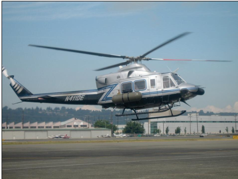
**Figure 7. AMS Bell 412 helicopter with externally mounted radiation detector pods.**
