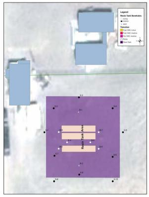
Figure 3. Resin Tank Sample Locations, B1- B8
