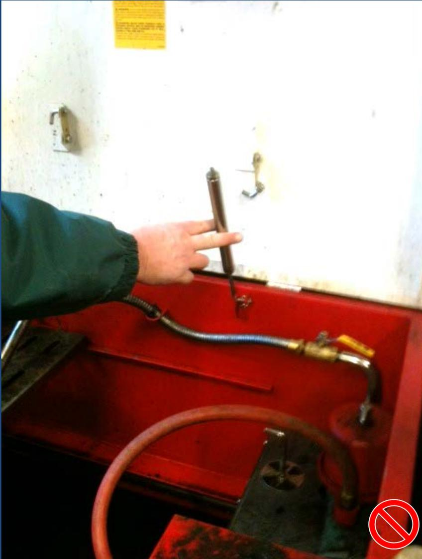
The fusible link system automatically closes the cover of the parts cleaner in the event that a fire occurs in the sink work area.
