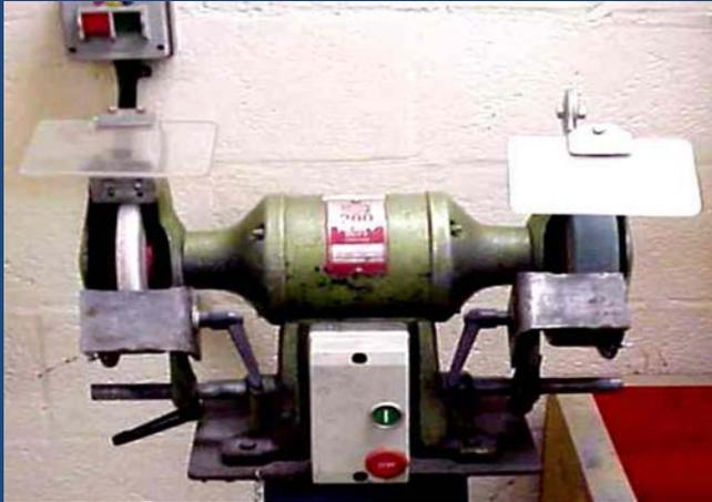
**Machinery with rotating or moving parts must have guards.**
