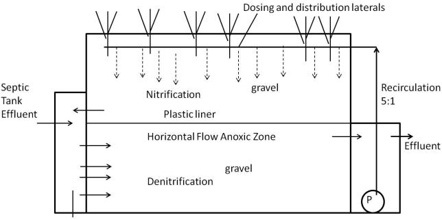
Figure A - 1 Vegetated Recirculating Gravel Filter (VRGF)
