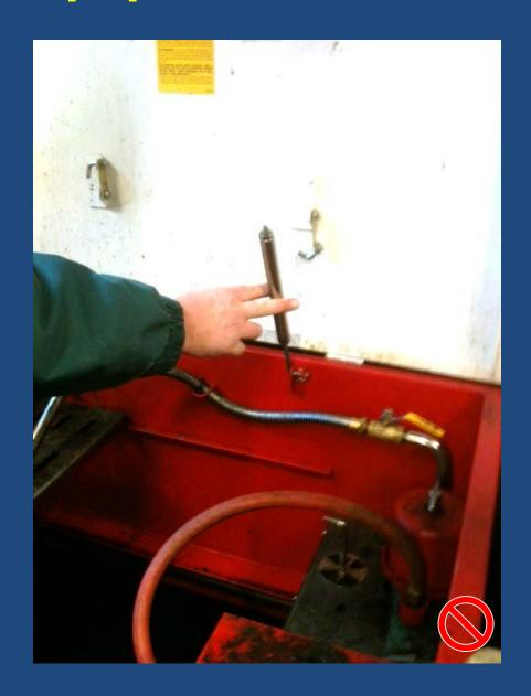
The fusible link system automatically closes the cover of the parts cleaner in the event that a fire occurs in the sink work area.
