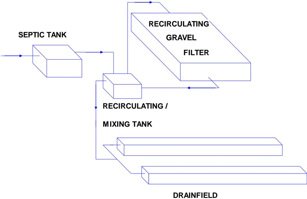
**Figure 2 – Cross-Section of a Typical Recirculating Gravel Filter**
