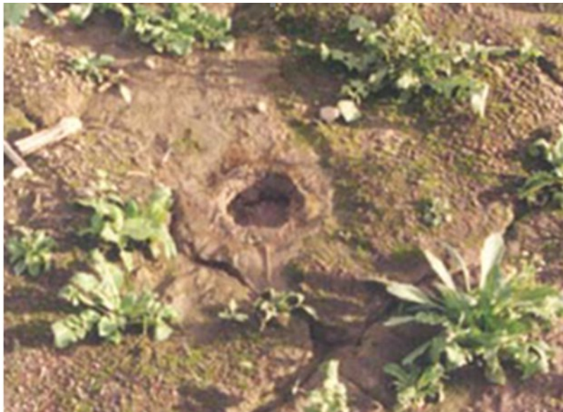
Figure 10. Example of Chimney Effect
