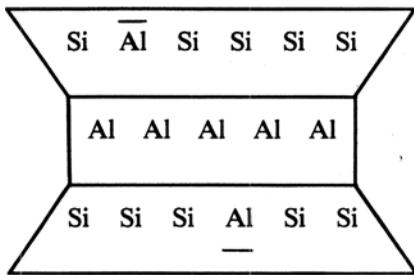
Fig. 1. Simplified structure of a silicate clay mineral, showing substitution in the silica layers and resulting negative charges on the surface. ( $O^{2-}$  and  $OH^-$  ions in the structure are not shown.)
