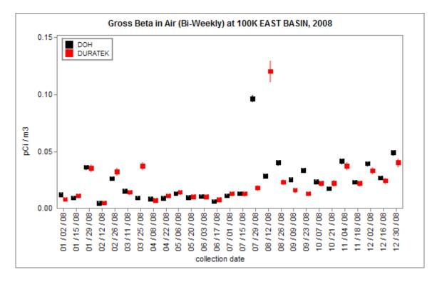
Figure 3.1.9 DOH and Duratek Gross Beta Concentrations in Air at 100K East Basin
