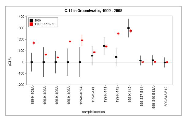
Figure 3.2.4 DOH and Fluor / PNNL Scatter Plot for Historical C-14 Concentrations in Groundwater
