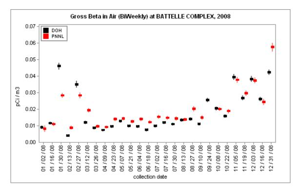
Figure 3.1.2 DOH and PNNL Gross Beta Concentrations in Air at Battelle Complex
