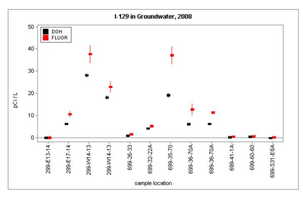
Figure 3.2.5 DOH and Fluor I-129 Concentrations in Groundwater
