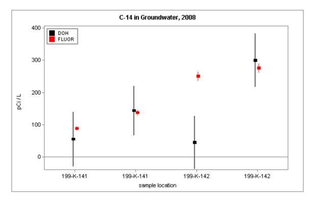
Figure 3.2.3 DOH and Fluor C-14 Concentrations in Groundwater
