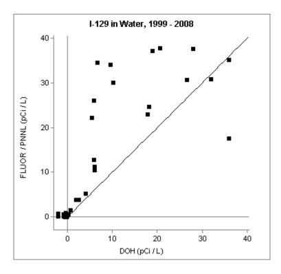
Figure 3.2.6 DOH and Fluor / PNNL Scatter Plot for Historical I-129 Concentrations in Groundwater
