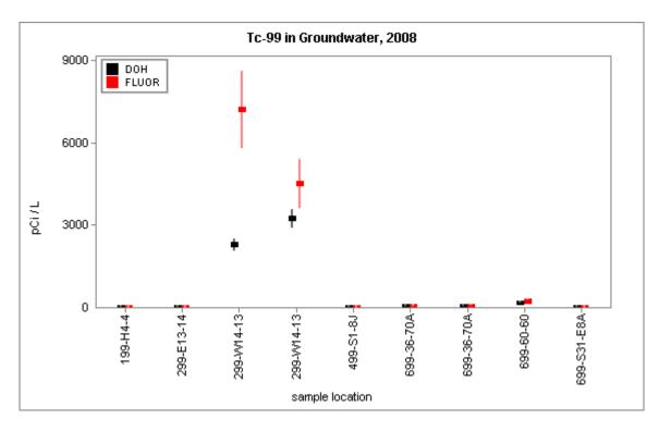
Figure 3.2.7 DOH and Fluor Tc-99 Concentrations in Groundwater
