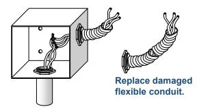
Replace the missing front panel of the electrical box and seal the small holes in the back.
