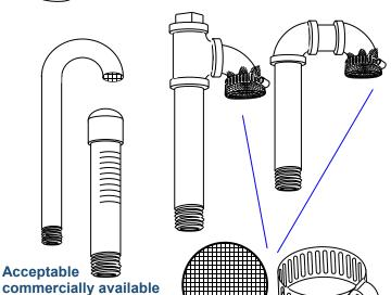
½-inch galvanized pipe with noncorrodible 24-mesh screen and a #12 stainless steel adjustable clamp
