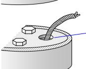
To seal the opening, remove the rope or attach it to an eyebolt on the sanitary seal bottom or drop pipe and use a square-head access plug. For a temporary fix, use clear silicone sealer around the opening.
