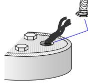
Install an electrical conduit to seal the opening around the wires on a submersible pump. For a temporary fix, use clear silicone sealer around the opening.
