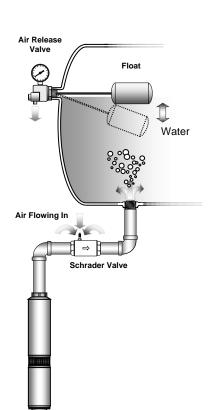
Another air charge system uses a **Schrader valve** to draw air into the line before the pressure tank. An air release valve discharges excess air from the tank. When a jet pump is used, the suction line introduces air into the tank through a snifter or Schrader valve.
