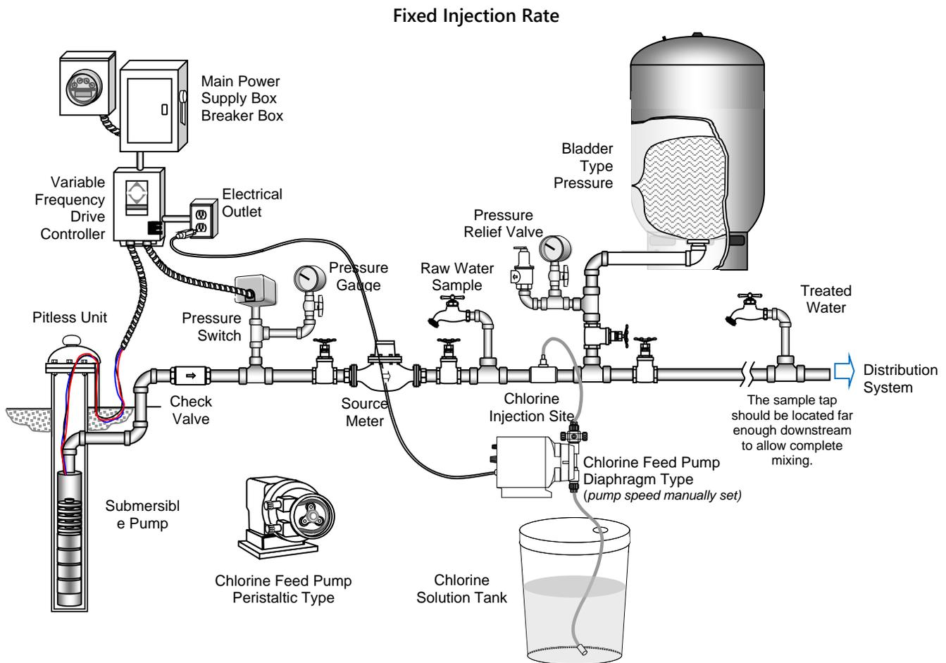
**Fixed Injection Rate—Pressure Switch.** The pressure switch turns the submersible well pump motor on and off. The pump control box turns the electrical outlet on and off at the same rate. When the system is operating, the water flow rate and the chlorinator output should be relatively constant. After mixing, the chlorine residual at the point of entry will be stable. Booster pumps can be controlled by pressure switches in the same way.
