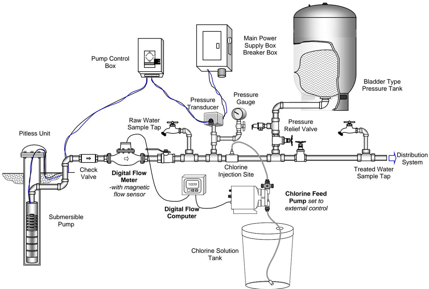
**Variable Injection Rate—Two Sources.** This water system has two well sources. They can operate alone or together, producing significantly different flow rates. The **digital flow meter** on the combined source water pipe keeps the output of the chlorine feed-pump proportionate to the water flow.
