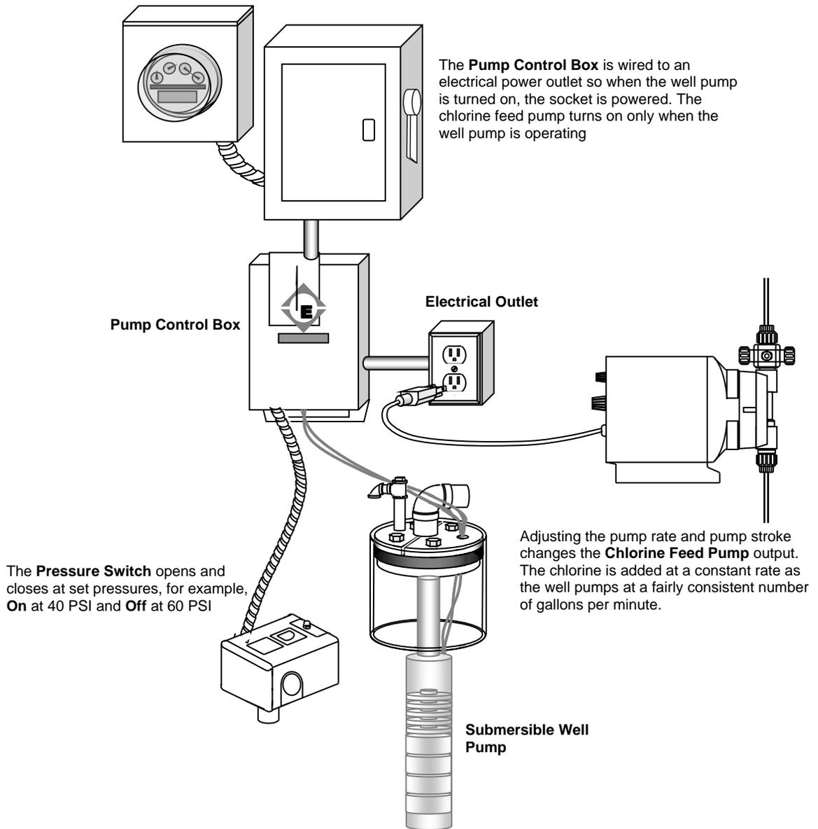
**Fixed Injection Rate—Reservoir Water Level Sensors.** Responding to a signal from the water level control box, the pump control box controls the electrical circuits for the chlorine feed pump and the well pump. When the well pumps water at a constant rate and the chlorine is added at a steady rate the resulting chlorine residual should be flow proportional.
