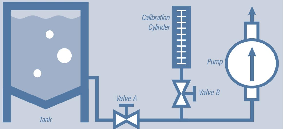
$$\text{Dose} \left( \frac{\text{mg}}{\text{L}} \right) = \frac{\text{Chemical Feed Rate} \left( \frac{\text{gal}}{\text{day}} \right) \times \text{Chemical Concentration} \left( \frac{\text{lb}}{\text{gal}} \right)}{\text{Plant Flow Rate (MGD)} \times 8.34 \left( \frac{\text{lb}}{\text{gal}} \right)}$$
