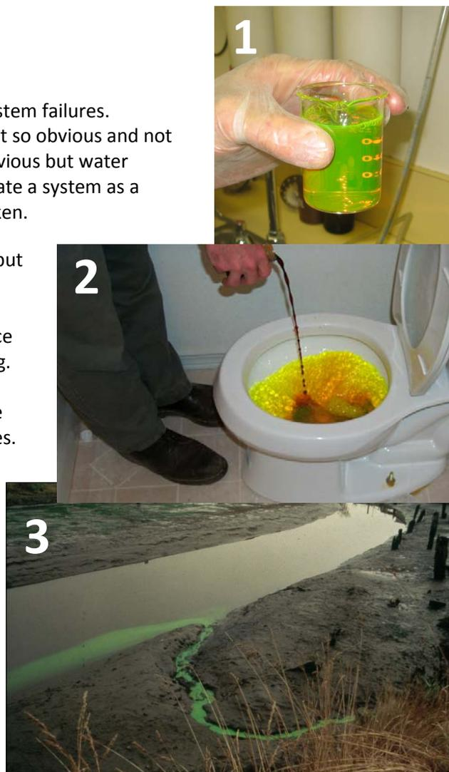
Figure 7. Photos illustrating the use and flow of fluorescence dye from the lab to the plumbing fixture to the environment.
