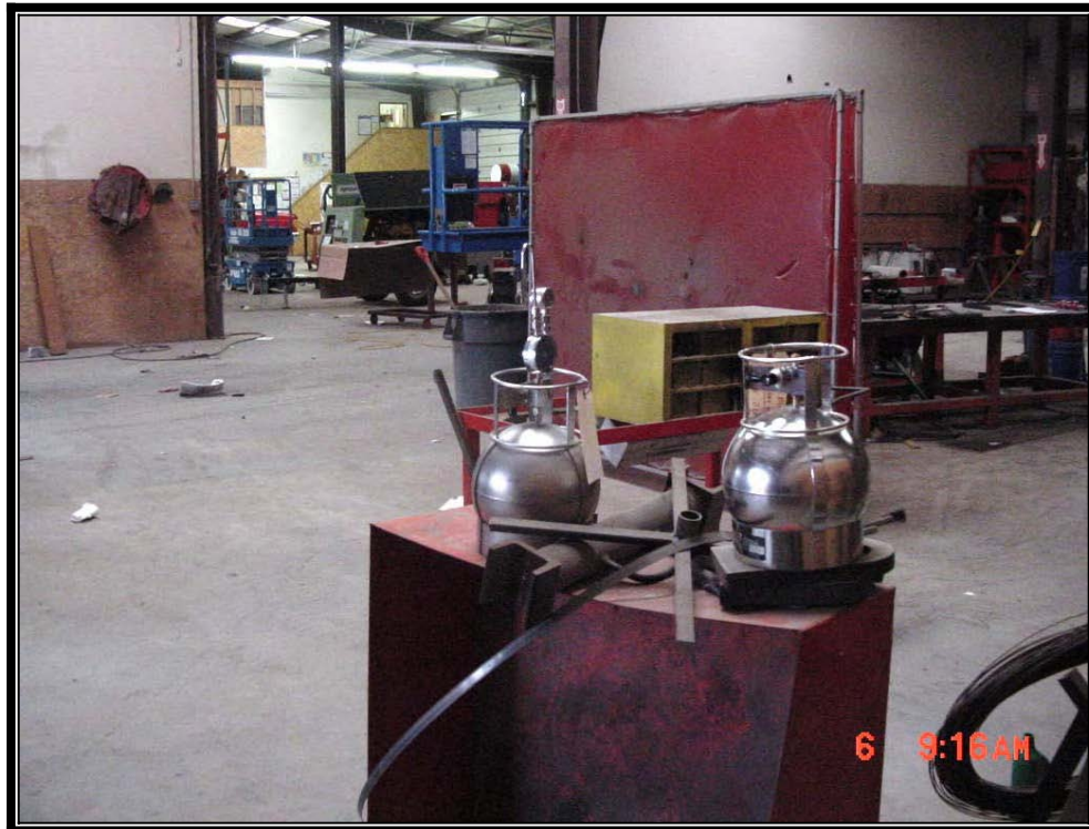
Photo 6. Air sampling (Summa) canisters
