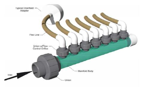
Figure 2. Typical Pressurized Flow Splitting Device
