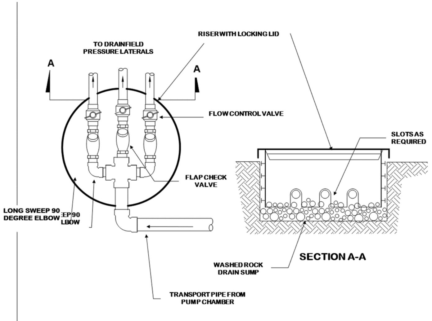
Figure 6B. Drainfield Control Box (Manifold Above Laterals)
