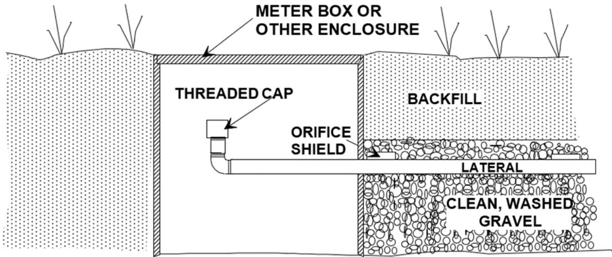
Figure 8B. Monitoring/Cleanout Port (Example). Cap must be secured.
