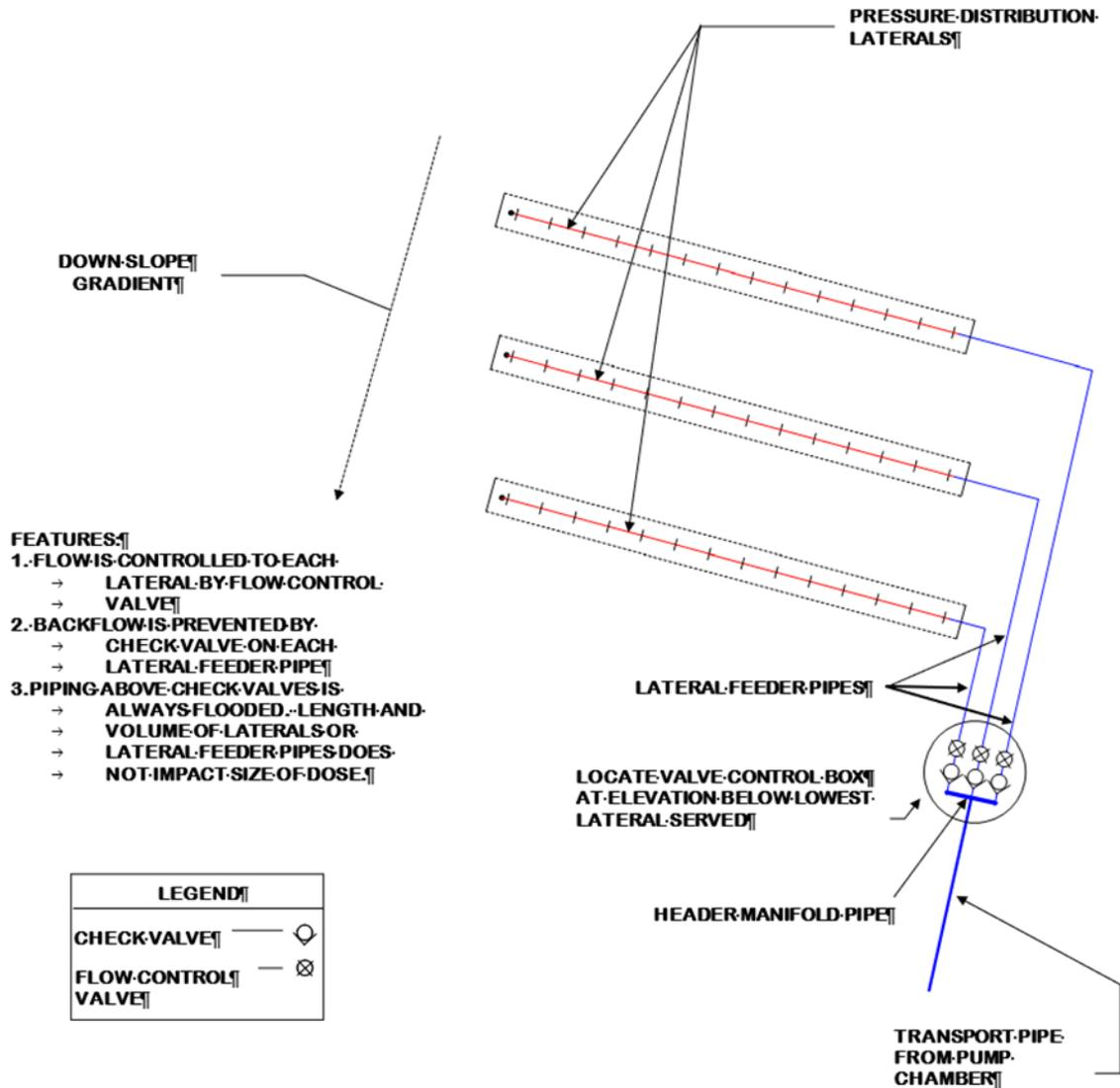
**Figure 3B. Pressure Distribution Drainfield (Sloping Ground, Manifold Below)**
