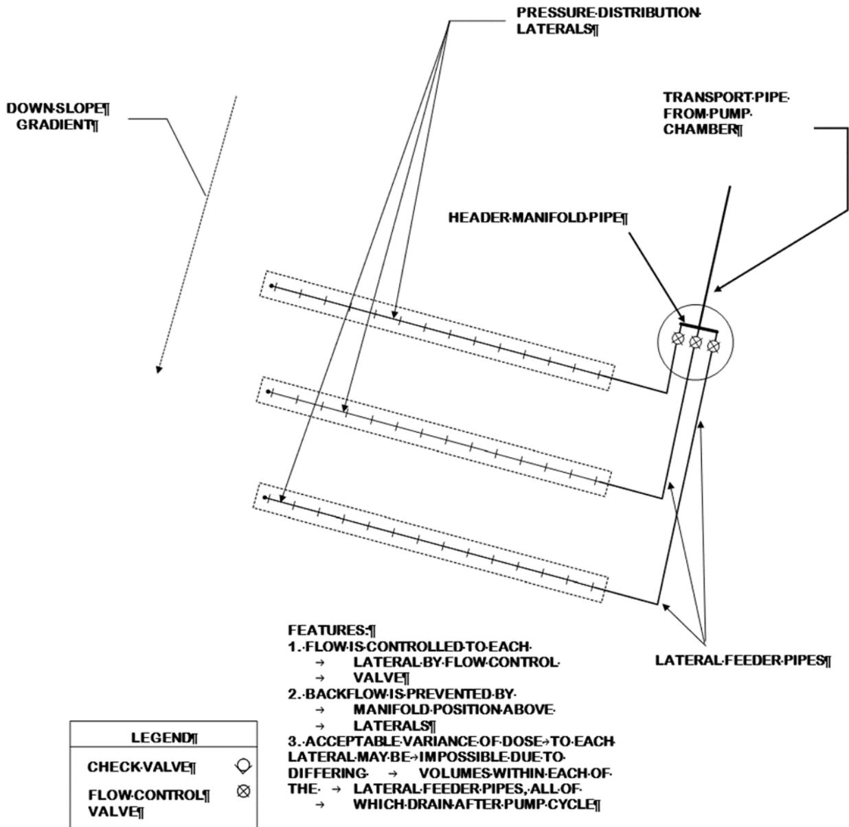
**Figure 4. Pressure Drainfield Cross Construction**
