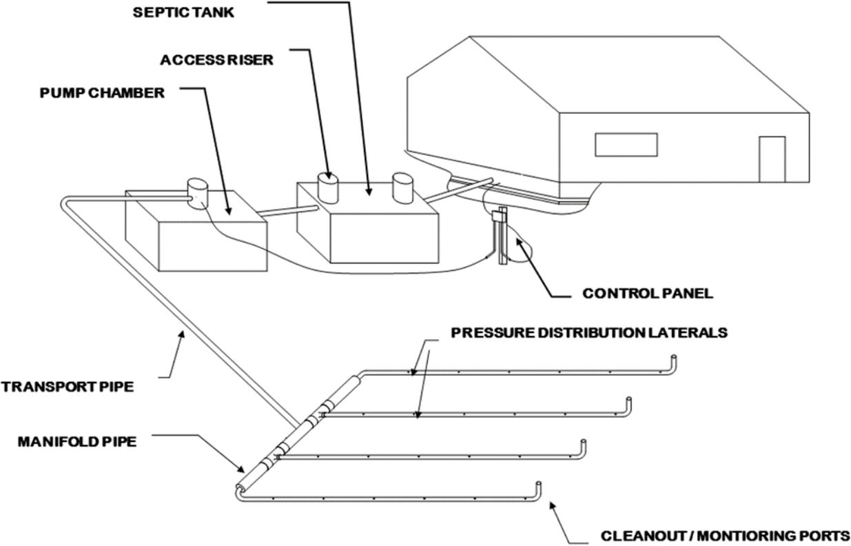
Figure 2. Typical Septic Tank and Pump Chamber
