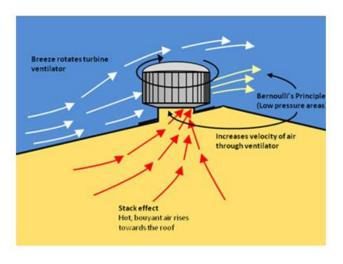
Field experience indicates that adding spinning barn vents – turbine ventilators- may aid in oxygen flow.
