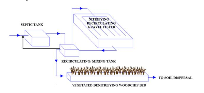
The recirculated effluent may be returned to either the recirculating mixing tank, the septic tank, or the sequence of the recirculation tank to the septic tank.
