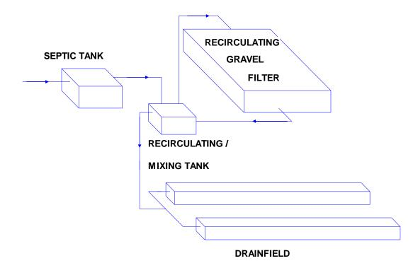
Figure 1 - Typical Layout of a Recirculating Gravel Filter
