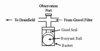
Tables 2 & 3 are provided as a guide in designing a recirculating ball valve. Actual inside diameters of the pipe and actual outside diameters of the ball must be used. The weight of the column of liquid in the return pipe must be overcome by the buoyant force of the ball. (Note: the weight of the sphere is neglected.) Density of effluent is assumed to be approximately 62.4 pounds/ft<sup>3</sup>.
