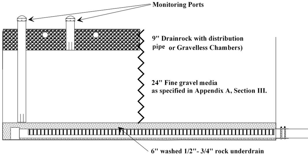
*Field experience indicates that adding vertical piping from the underdrain to the surface may help with rehabilitation of failed filters. Spinning barn vents (turbine ventilator) may aid in oxygen flow.*
