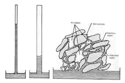
Upward movement by capillarity in glass tubes as compared with soils (after Brady<sup>10</sup>).
