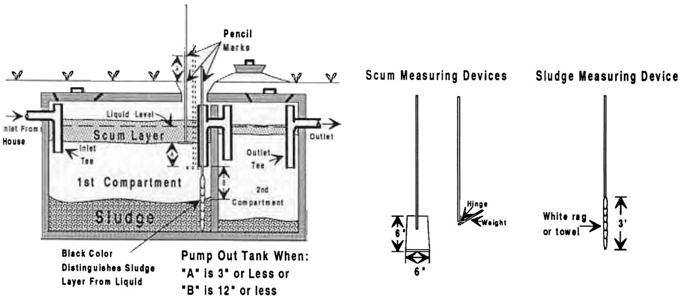
If a filter is installed on the outlet of the septic tank, it should be cleaned whenever the tank is inspected. Pump chambers should be checked regularly for accumulation of solids on the floats, proper function of the alarm system, pump operation within the designed pumping period, and evidence of water infiltration. Drainfields should be inspected for surfacing moisture, lush growth of plants, and odors. Septic tank additives are of no known value and some can be very harmful
