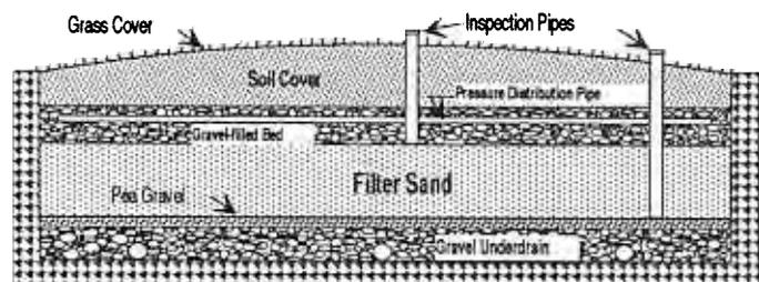
the bottom and sending it to disposal. The effluent from a sand filter must still be discharged to a subsurface soil absorption system. A special type of sand filter is a sand-lined trench or bed. For these special sand filters, the filtrate is not collected for disposal, but instead infiltrates into the soil at the bottom of the trench. These systems provide a high degree of treatment of BOD, TSS, microorganisms, and some nitrate reduction.
