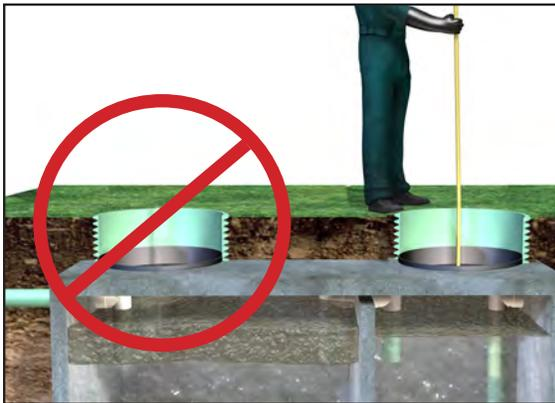
*KEEP TANK OPENINGS IN FRONT OF YOU. FALLS MAY OCCUR WHEN PEOPLE STEP BACKWARD INTO AN OPEN TANK. NEVER LEAVE AN OPEN TANK UNATTENDED.*
