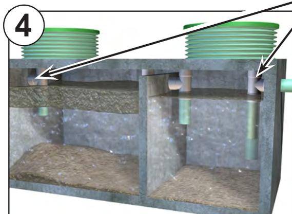
Are baffles free of clogs and leaks around the seals to the tank? If the baffle is concrete, is it intact and not corroded?
