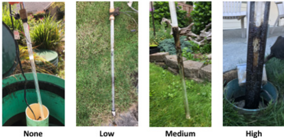
Figure 4. Rankings of Biofilm Deposit on UVD Unit Protective Sleeves
