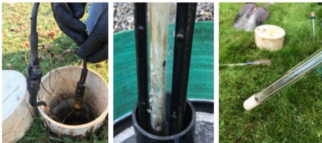
Figure 7. Examples of Common UVD Unit Issues. From left to right: electrical corrosion, torn Teflon sleeve, and water intrusion.
