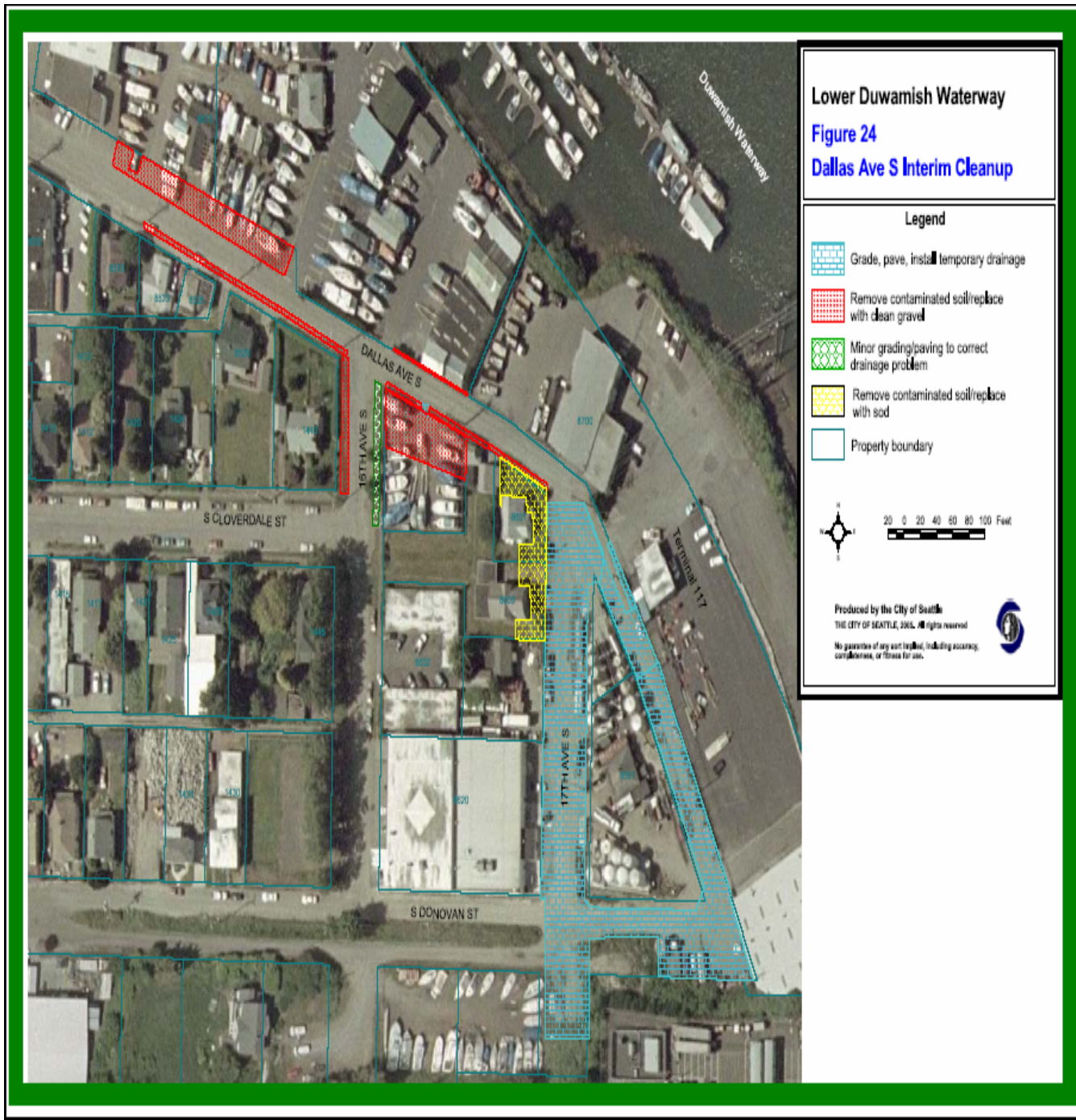
Figure 5 – Street/Yard Soil Interim Cleanup, Locations: Dallas Avenue South Soil Removal Site Seattle, Washington
